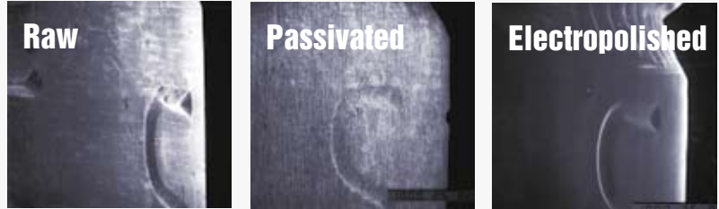
After 2560 hours salt spray - Passivated (left), Electropolished (right).
