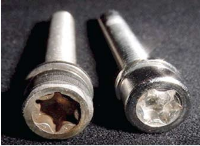
After 2560 hours salt spray - Passivated (left), Electropolished (right).
