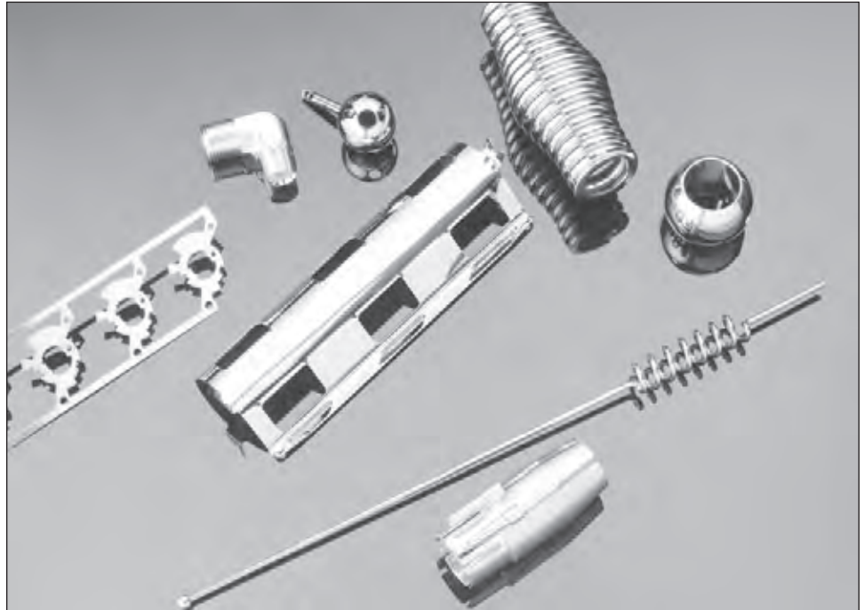
Many parts are sized through electropolishing. Virtually all alloys including carbon steel, brass, aluminum, copper, Inconel, Monel, Hastelloy, molybdenum and stainless steel are successfully electropolished.
