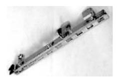
**Solution:** After electropolishing samples, processing parameters were established. The parts were tested for corrosion resistance and exceeded part specifications. During continued use, the parts withstood the effects of harsh cleaning solvents. In addition, the electropolishing enhanced the microfinish which reduced product buildup and shortened the cleanup time.
