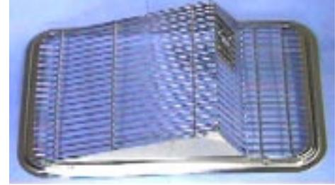
**Solution:** Electropolishing removed the surface metal and eliminated the weld discoloration. Being an electrochemical process, all surfaces were processed simultaneously, allowing for a uniform finish at low relative cost. Most importantly, the assembly was highly corrosion resistant, exceeding customer specifications.
