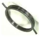
**Solution:** Electropolishing eliminated the stress points in the wire. After removing .0005 to .001 material, the parts exceeded the cycle life requirement. Raw springs reached 147,000 cycles. Electropolished springs reached 800,000 cycles. As surface metal was dissolved, so was the heat tint caused by the heat treat operation.
