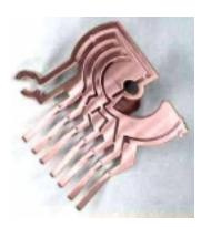
**Solution:** Electropolishing removed the burrs, and in the process made the part's surface smoother, easing assembly. This was achieved without incurring any damage to the fragile fingers.
