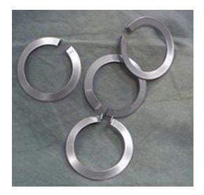
**Solution:** Able electropolished the 316 stainless steel to a bright finish. We concentrate on the critical reflective surface. The reflection rings are carefully handled and placed into individual plastic auto bags. Able Electropolishing has been processing this part continuously for over ten years.
