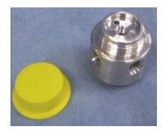
**Solution**: Able® electropolished the regulator body by removing a precise amount of metal. The corrosion resistance is greatly improved and surface finish was improved by as much as fifty percent. The part was cleaned, brightened, and fully passivated in one operation. The customer required fully cleaned ports and holes with no visible evidence of oxides or discoloration. Able also provided special packaging for each part.
