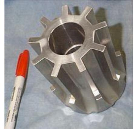
**Solution:** Our customer decided to try machining then electropolishing the 'Extruding Head'. We electropolished several control samples and the results looked promising. The end customer tested the new design in their ice making equipment. The tests were successful. The end customer had a part that went from several costly uncontrollable steps down to two: machining and electropolishing. Electropolishing provided a smooth, bright passive, defect free surface all in one low cost operation.
