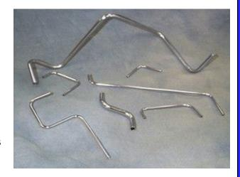
**Solution:** Our customer began by electropolishing a group of samples. By removing a controlled amount of metal from the surface, all oxides and imbedded impurities were removed. Able Electropolishing was called upon to provide a clean and bright finish. The outside surfaces are electropolished while the inside surfaces are fully passivated. Since there are no coatings to chip or peel, the bright finish will last for years, even in an oceanic environment.
