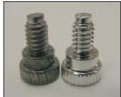
Scale and discoloration are removed without thread damage.
